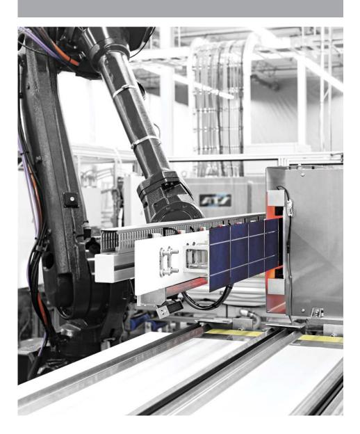
Producing high quality modules requires precision handling and placement of cells and strings; combined with in process inspections, the ATS Solstice™ String & Layup station uses industry standard stringers coupled with our virtually break-free layup to produce best-in-class modules
