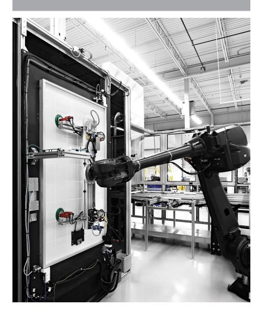
**///** Maximized revenue generation comes from accurately rated modules. The ATS Solstice<sup>™</sup> PV Measurement System helps achieve this by using an optimized combination of light source, instrumentation, and intelligent software, with testing at the cell or module level.
